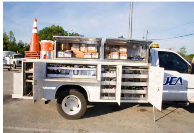
After 5S: Tools Sorted, Organized, and Stored in Labeled Compartments on the Water Maintenance Truck
